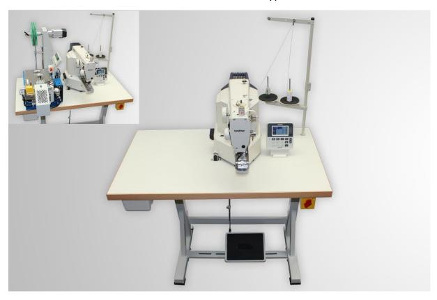
This automatic bartacker can be placed directly next to the lifttape cutter to ensure a continuous and smooth production flow.
