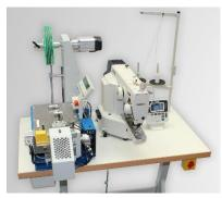
If the lifttape cutter and automatic bartacker are combined at one workstation, a touch panel with integrated PC can be connected to the cutting machine as an expandable option. With this PC, different jobs can be stored or read in and quickly retrieved. This increases productivity and efficiency.
