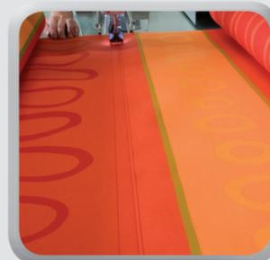
With the Sewsy™ the sewing head moves while the material is held still, resulting in perfectly straight seams with consistent overlap.
