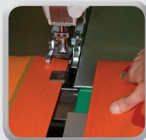
Fabric panels are clamped and start and end and remain perfectly aligned during the entire sewing cycle.
