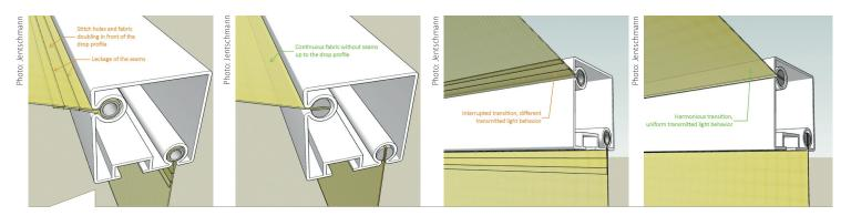
Since the new production technique eliminates the sewn fabric fold-over at the front profile, there are no more problems with leaking seams in this area.
