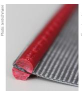
The piping, which is mechanically halved and sewn through the fabric, creates a "seamless" transition to the fabric, meaning that the otherwise customary fabric fold-over can be dispensed with during fabrication.
